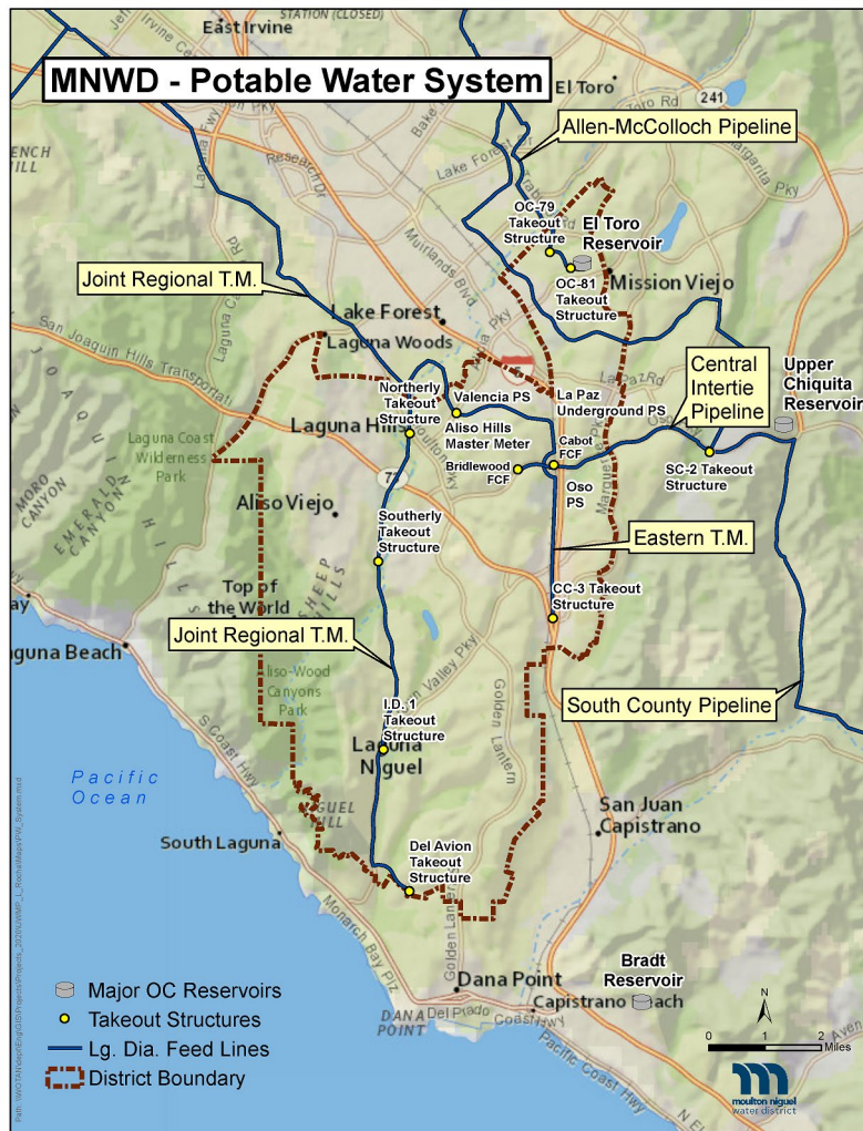
Figure 1-2. MNWD Potable Water System
