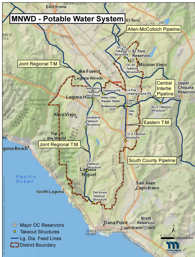
Figure 1-2. MNWD Potable Water System
