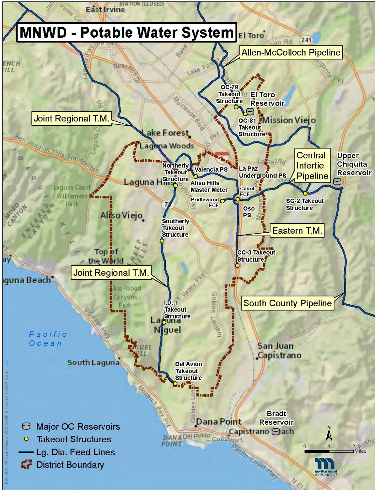
Figure 3-3: Potable Water System
