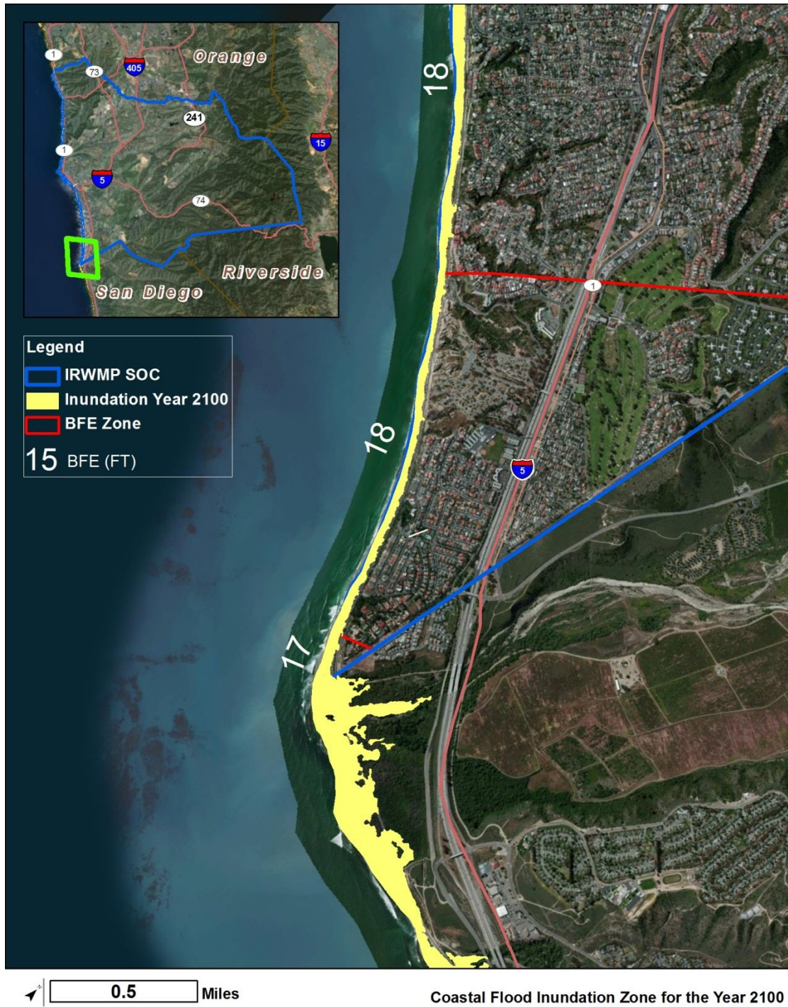
Figure 7-12 Zoomed-in area of South OC coastline, zone 6, identifying areas (in yellow) that are under flooding threat due to the combined effects of a 100-year flood and sea-level rise to 2100 (55 inches). Numbers along the coastline are FEMA's BFE values in feet.
