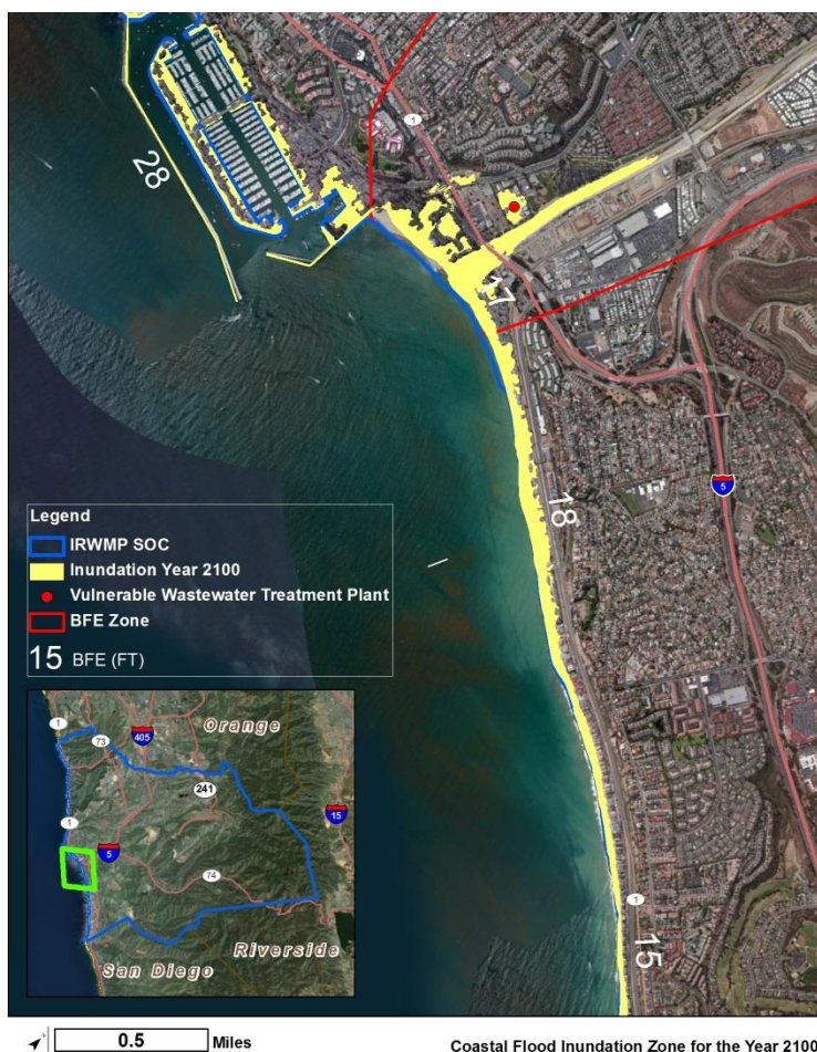
Figure ES-1. Zoomed-in area of South OC coastline, identifying areas (in yellow) that are under flooding threat due to the combined effects of a 100-year flood and sea-level rise to 2100 (55 inches). Numbers along the coastline are FEMA's base flood elevation values in feet.
