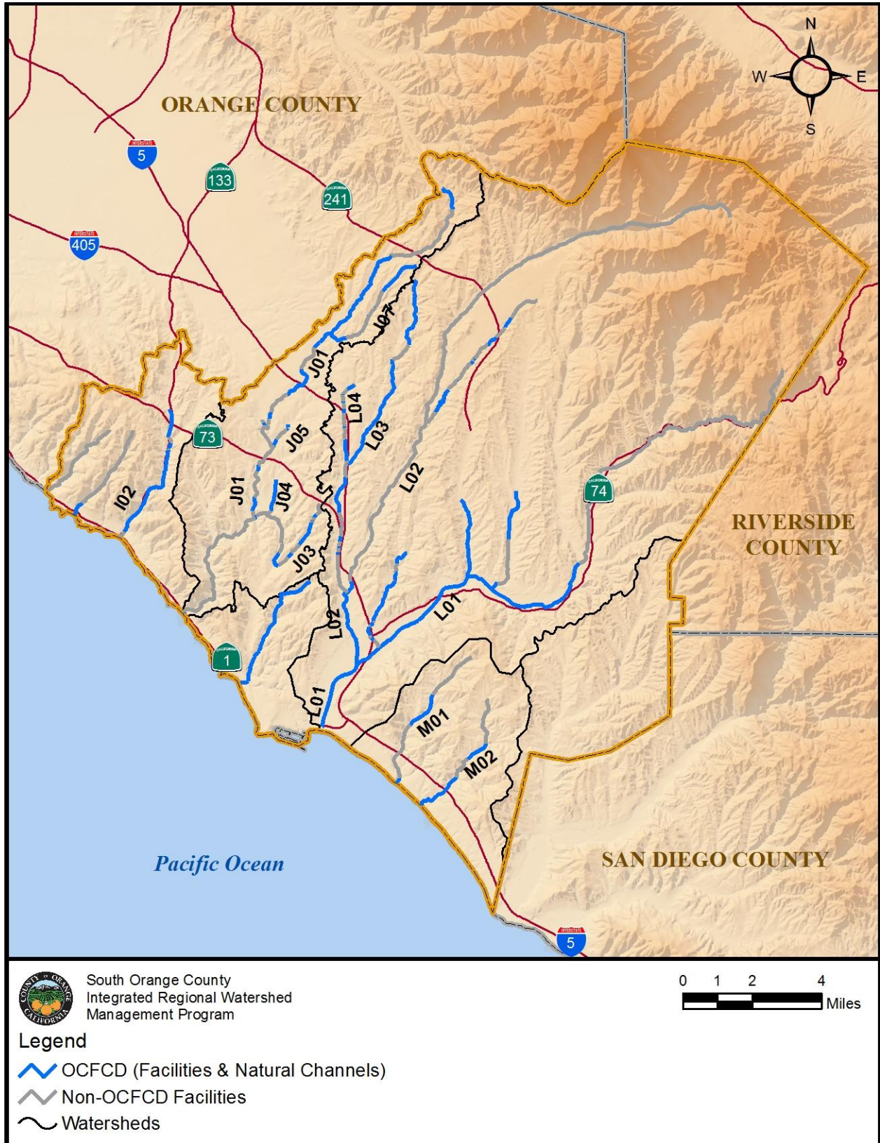
Figure 3-11: Flood Control Infrastructure
