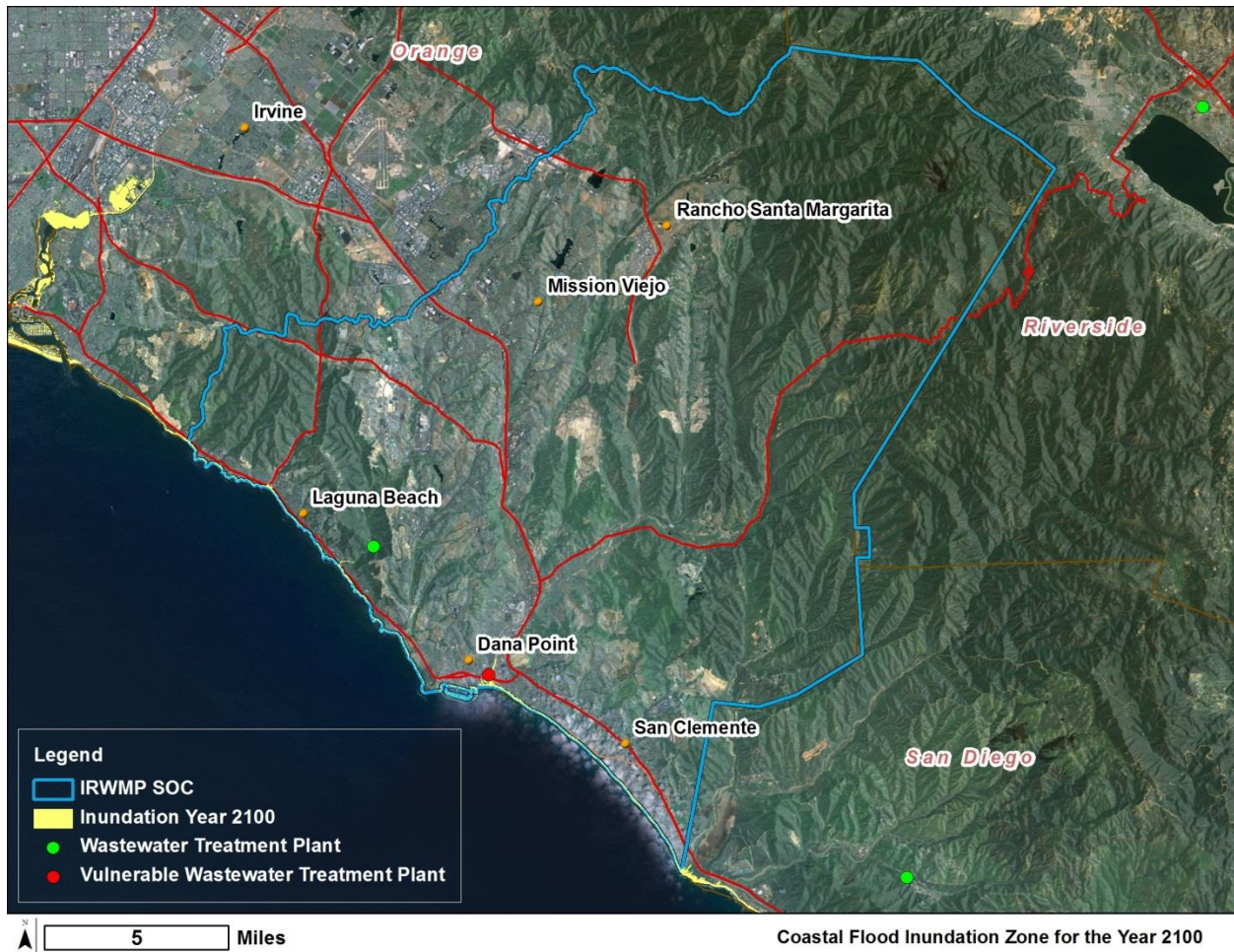
Figure 7-6 Projected inundation areas (in yellow) corresponding to a 55-inch rise in sea-level along South OC. The areas of inundation in this region occur along a narrow strip along the coastline and do not extend inland. There is a vulnerable wastewater treatment plant near Dana Point that is identified on the map.
