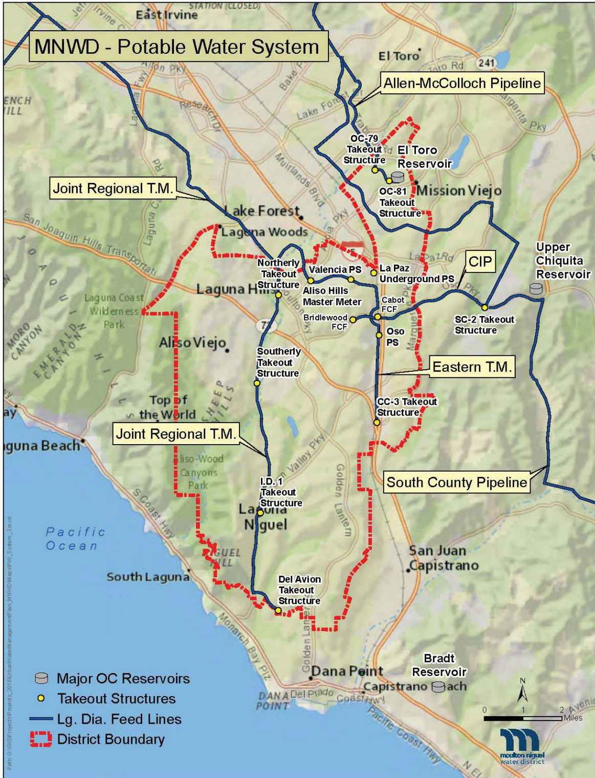
Figure 2-2: MNWD - Potable Water System
