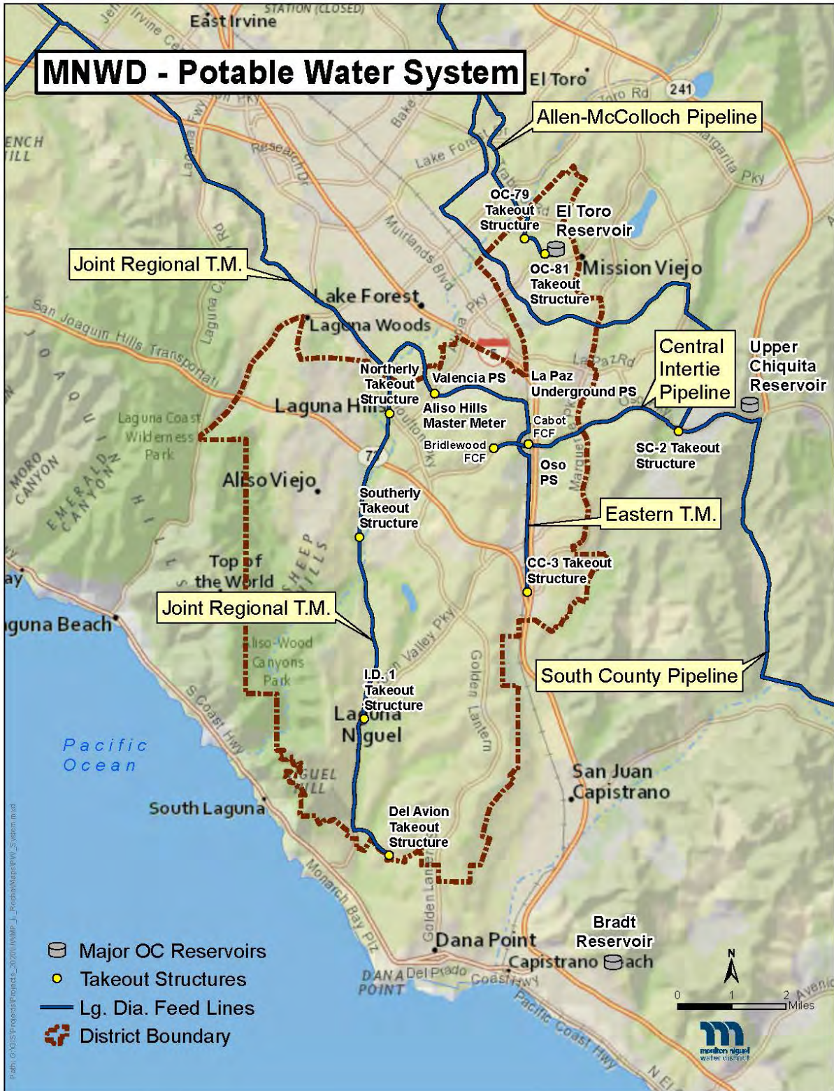
Figure 3-3: Potable Water System
