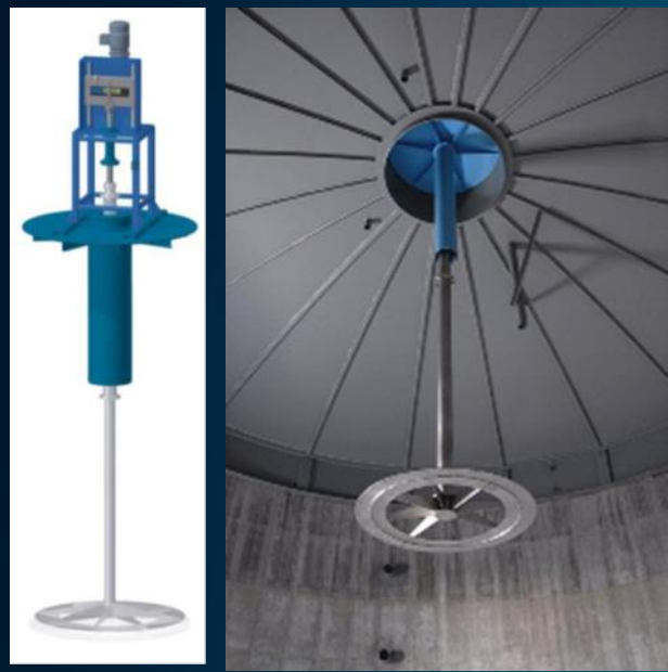
Linear Motion Digester Mixing
