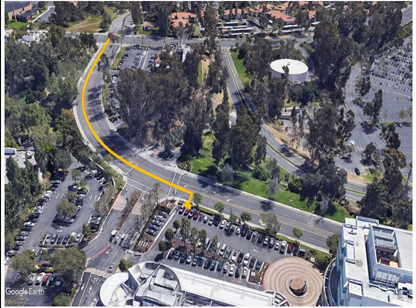
Alignment of New 12-inch PVC Mainline
