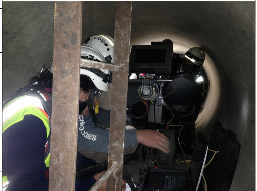
Electromagnetic Inspection of the Central Intertie Pipeline
