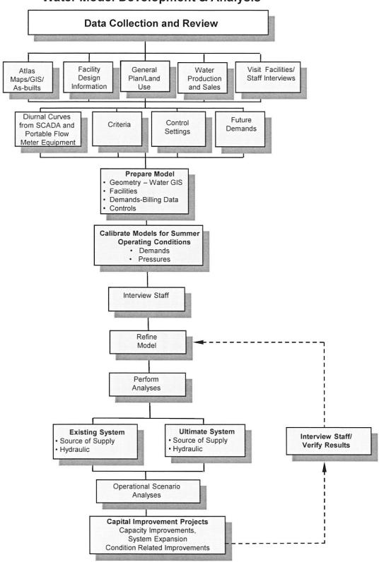
Linking the water billing data to the water meter shapefile will allow us to use the meter data to obtain a very accurate spatial distribution of demands. Meter consumption data will be adjusted to match the established existing low period, average day and maximum day demands.
